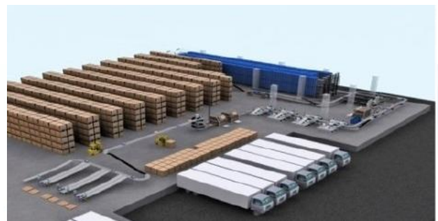
Automated Logistics Facility: 20,000sq m high-tech automation facility featuring 12,000 tote multi-shuttle system from Dematic.
